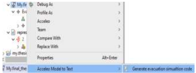
Fig. 6. Running the Aceleo code as a context menu on the model file
