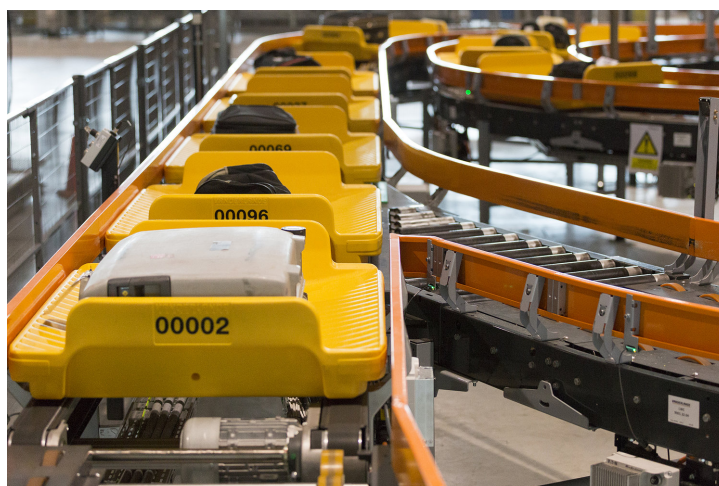
Figure 1.3: Yellow carriers with baggage used in the Tubtrax system.
