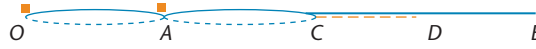
Figure 1. Counterexample of the concatenation of shortest paths. The squares represent the gauge changeovers, the solid line represents the Iberian gauge line, the dashed line represents the standard gauge line and the double line (solid and dashed) represents the mixed gauge section.
