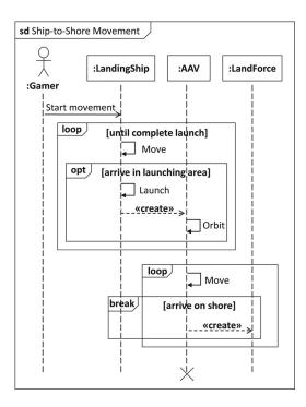
Fig. 12. Sequence diagram for ship-to-shore movement.
