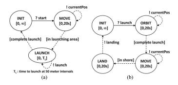
Fig. 15. DEVS diagram for landing ship and AAV. (a) Landing ship. (b) AAV.
