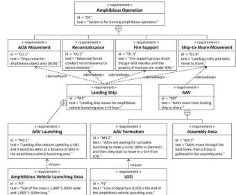
Fig. 10. Requirements diagram for amphibious operation system.
