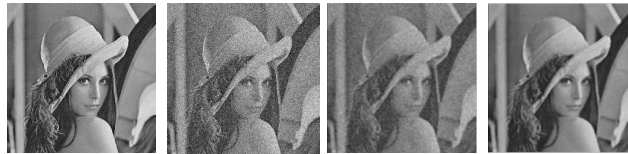
Figure 5. Application of the 30 % CA filter on the Lena image.
