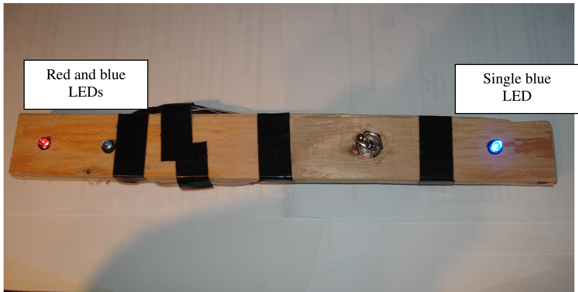
Figure 5-16: Alternative more manoeuvrable stereo calibration stick
