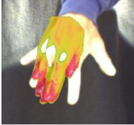
Figure 4-28: Incorrect selection of initial IR/IO image frames for overlay
