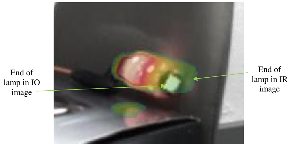
Figure 5-14: A small object rotation causes a misalignment at an angle of 50°
