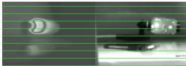
Figure 5-15: An example of epiline alignment for the 50° angle case when the object is aligned directly in front of the two cameras.
