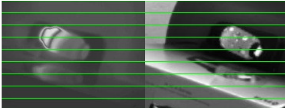
Figure 5-11: Rectified IR & IO images for experiment 3 with a relative camera angle of 10^\circ
