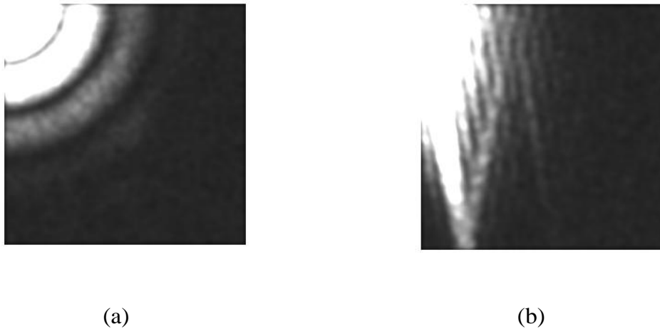
Figure 3.14: Low pass filtered DCT spectrums of an image degraded by out-of-focus and motion blur.
