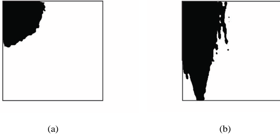
Figure 3.15: Low pass filtered DCT spectrums of an image degraded by out-of-focus and motion blur is transferred to binary domain using a suitable threshold.
