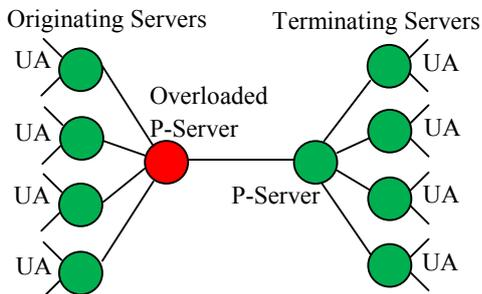
Fig. 3. SIP network topology with an overloaded P-server (which is marked in red color) and its multiple upstream originating servers
