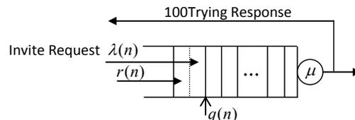
Fig. 4. Queuing dynamics of an overloaded SIP server ( $\lambda(n)$  denotes aggregated original message arrivals,  $r(n)$  denotes aggregated retransmitted message arrivals from multiple upstream servers,  $q(n)$  denotes queue size,  $\mu(n)$  denotes service rate)
