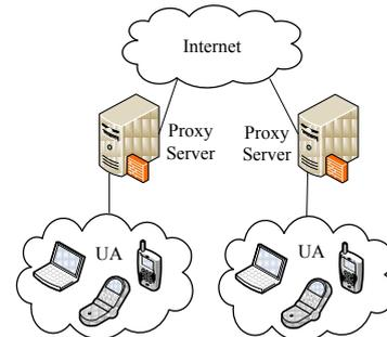
Fig. 1. Simplified configuration of a SIP network
