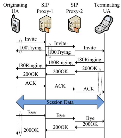
Fig. 2. A typical procedure of session establishment
