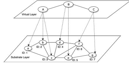
Fig. 1: An example of VNE with its associated substrate network.
