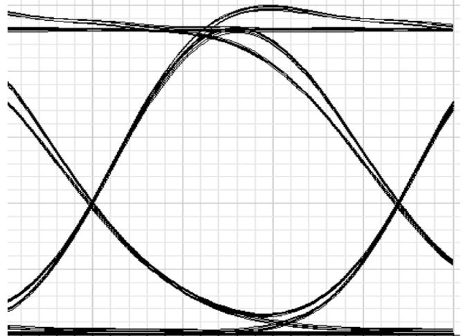
(vi.) MetroCor length 300 km, signal power 10 dBm, quality factor 3.70359 and BER  $9.68246e-005$  when data rate is 65 Gbps.
