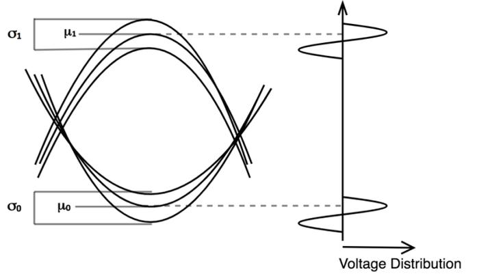
Fig 3. Mean values and standard deviation of the eye diagram having voltage distribution as measure of power.
