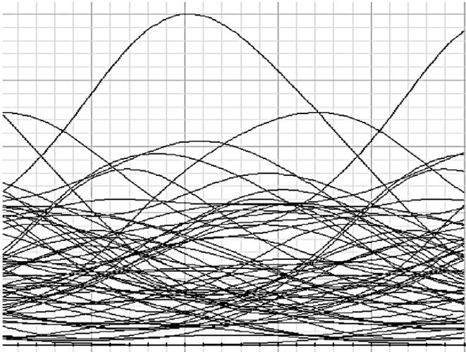
(vii.) SMF-28 length 300 km, signal power 0 dBm, quality factor 0 and BER 1 when bit rate is 65 Gbps.
