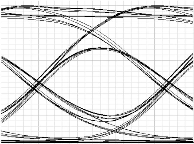
(i.) MetroCor length 300 km, signal power of 0 dBm produces quality factor 4.122 and BER  $1.803e-0050$  when data rate is 95 Gbps
