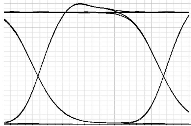
(ii.) MetroCor length 300 km, signal power of 0 dBm, quality factor 54.05 and BER 0 when data rate is 35 Gbps. This is the most desired implementation as there is highest Q-Factor and minimum errors.
