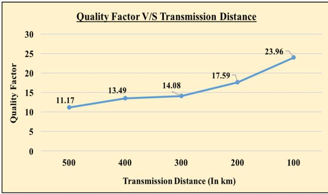
Chart 2. Quality Factor V/S Transmission Distance for constant data rate (65 GBPS) and power (0 dBm). Quality factor is improved with reduction in the transmission distance.
