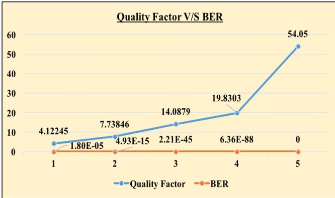
Chart 3. Quality Factor V/S BER with consistent transmission distance (300 km) and power (0 dBm). Efficiency improves with lower BER.
