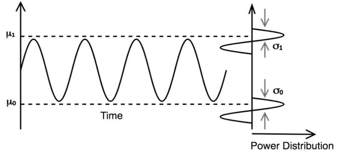
Fig 2. Mean values and standard deviation of the signal with respect to time and power distribution.
