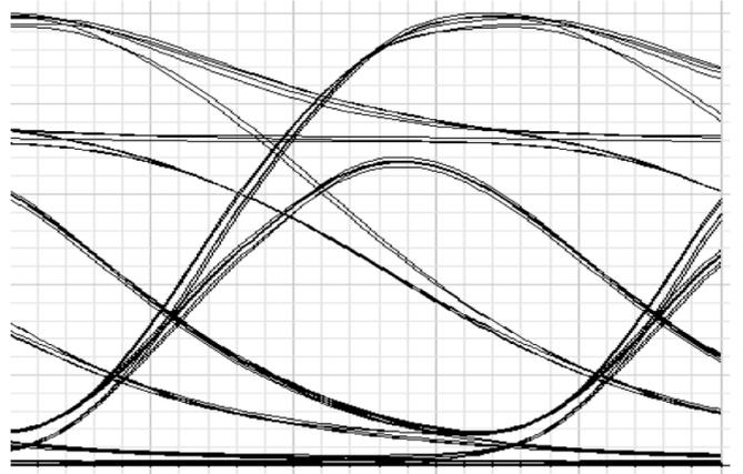
(v.) MetroCor length 300 km, signal power -10 dBm, quality factor 15.182 and BER  $2.1964e-052$  when data rate is 65 Gbps.
