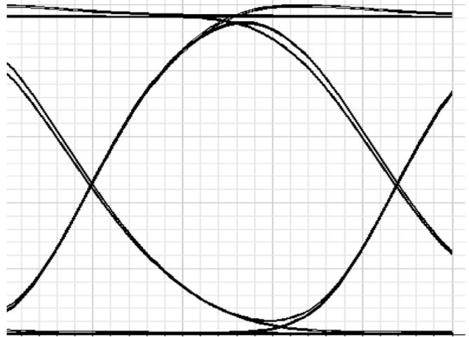
(iv.) MetroCor length 100 km, power 0 dBm, quality factor 23.9681 and BER  $2.9523e-127$  when data rate is 65 Gbps.
