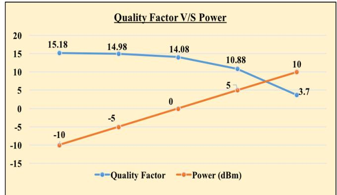
Chart 6. Quality Factor V/S Power transmission for steady distance (300 km) and data rate (65 GBPS). With expansion in transmitting power the quality factor is depleted.
