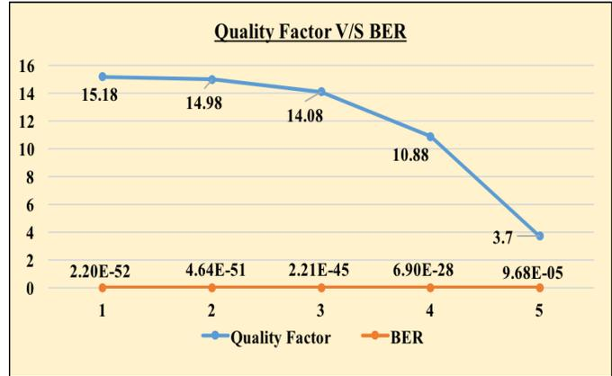
Chart 5. Quality Factor V/S BER for steady transmission distance (300 km) and data rate (65 GBPS). Reduction in quality factor with gain in BER is observed.
