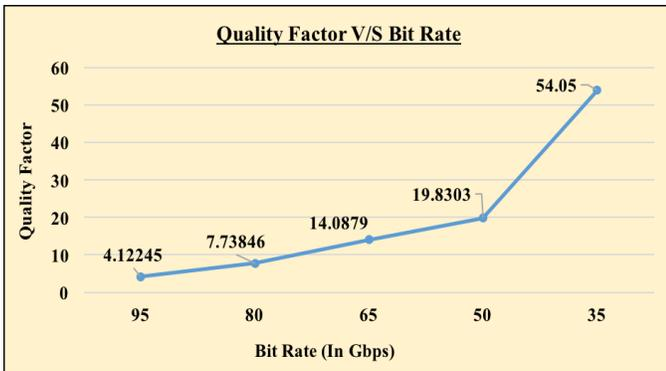
Chart 4. Quality Factor V/S Bit Rate with consistent transmission distance (300 km) and power (0 dBm). With higher data rates there is depletion in productivity.
