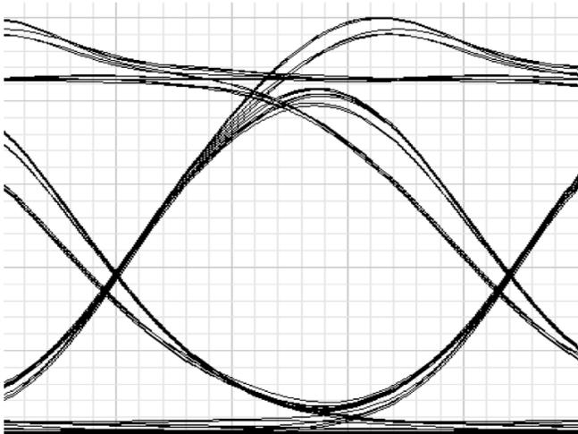
(iii.) MetroCor length 500 km, signal power 0 dBm gives quality factor 11.1775 and BER  $2.60466e-029$  when data rate is 65 Gbps.
