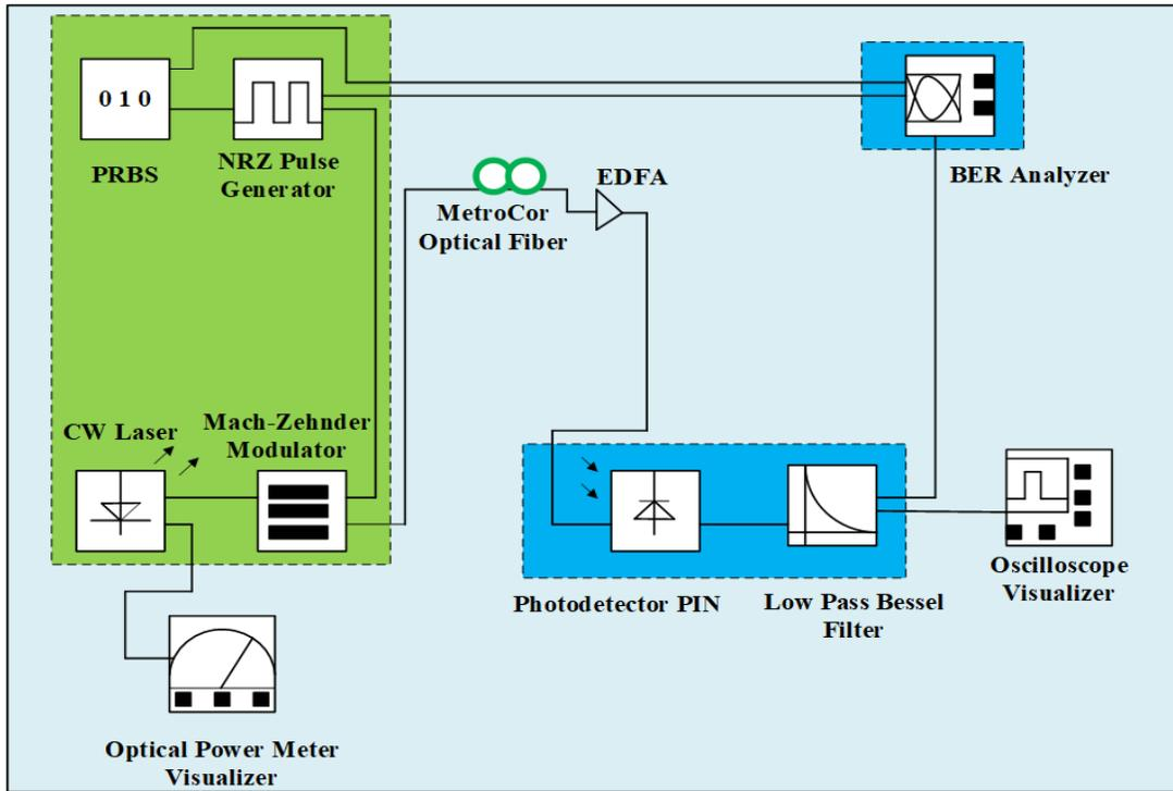
Fig 1. Simulation setup of the optical telemetry. Transmitter section is in green whereas the receiver part is in blue background.
