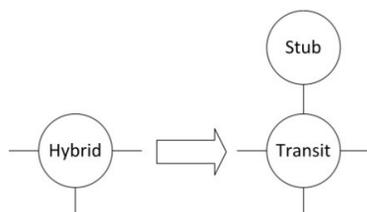
Fig. 1. Illustration of decomposing a hybrid node into a transit node attached with a stub node.
