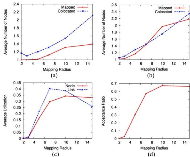
Fig. 11. Results with heterogeneous nodes: (a) average number of SSNs a VSN mapped onto and average number of collocated VSNs; (b) average number of STNs a VTN mapped onto and average number of collocated VTNs; (c) average CPU utilization of sub substrate nodes and average link utilization of substrate links; (d) acceptance ratio.
