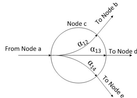
Fig. 7. An illustration on how traffic from a virtual link  $(a, c)$  is split into three output streams within VTN  $c$ .
