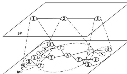
Fig. 2. Modeling MapReduce computation with virtual nodes. S stands for servers; T stands for Top of Rack switch; A stands for aggregation switch.
