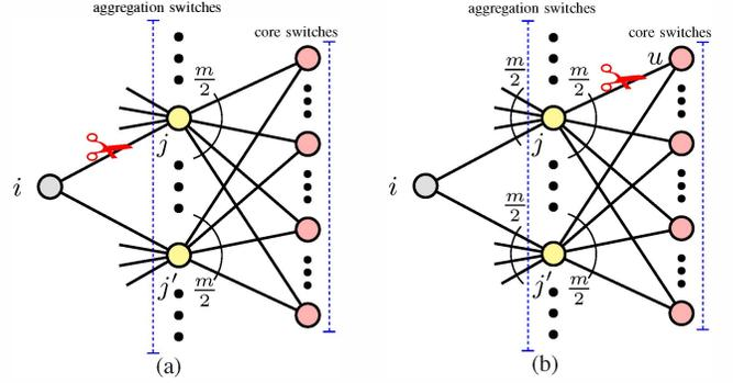
Fig. 3. Single link failure on VL2. (a) A failed edge link. (b) A failed core link.
