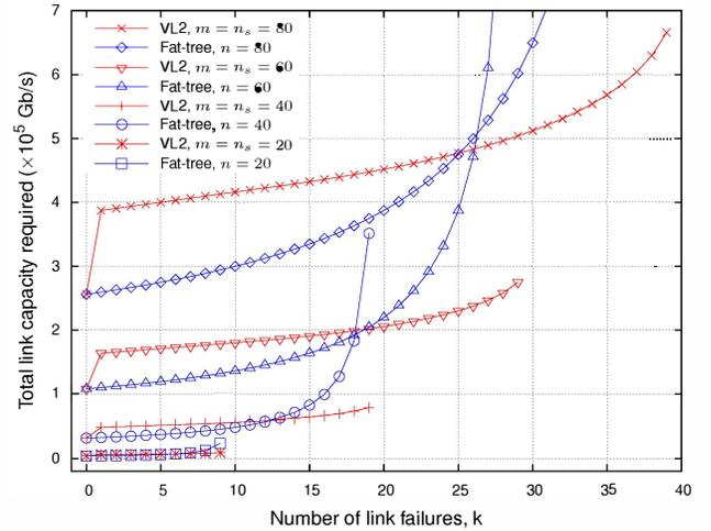
Fig. 5. Total link capacity comparison between VL2 and fat-tree.
