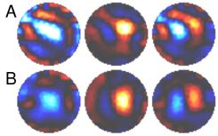
EIT images in anaesthetised, ventilated dog A: uncompensated, B: compensated. *Left*: ventilation *Centre*: saline (right lung) *Right*: ventilation and saline
