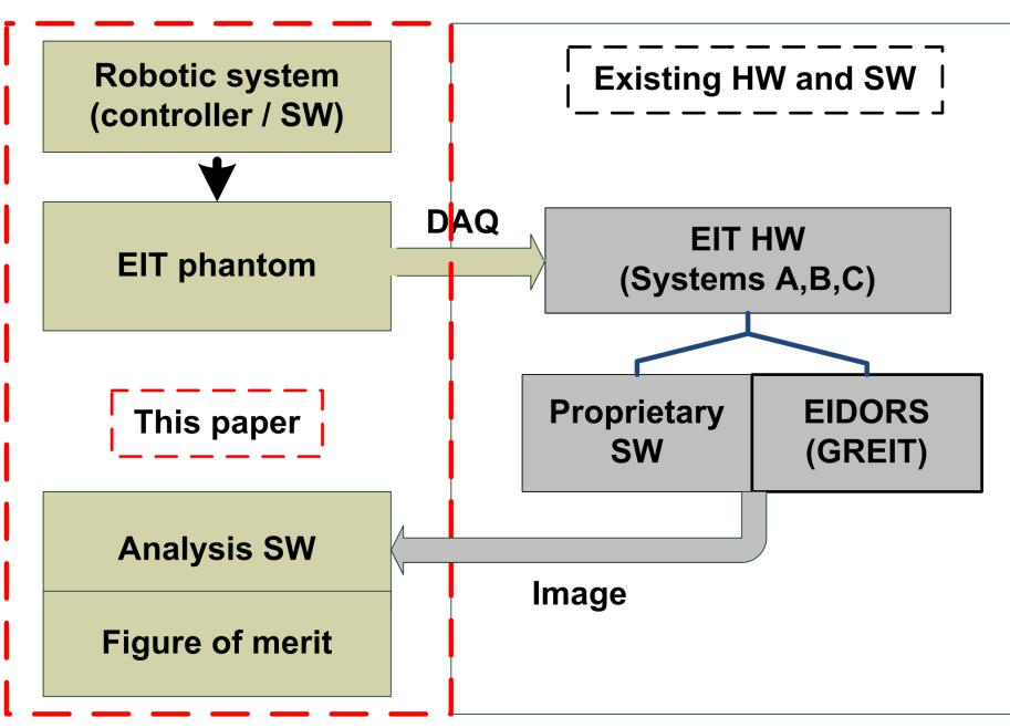
A phantom test system was constructed using a robot, saline tank phantom, test targets and EIT measurement system. We have carefully calibrated resistive targets.
