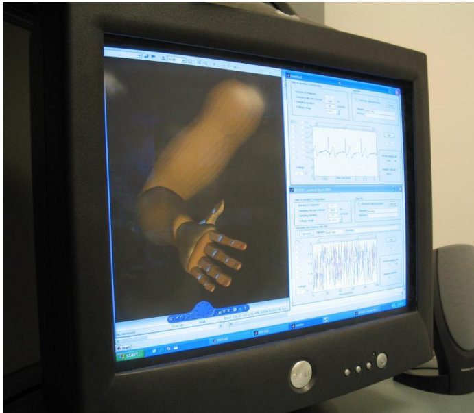
Virtual Arm controlled by muscle signals
