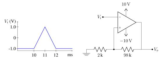
Sketch  $V_+$  and output  $V_o$ . Show voltage levels and the times of any transitions. (Assume op amps are ideal)
