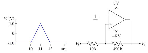
Sketch  $V_+$  and output  $V_o$ . Show voltage levels and the times of any transitions. (Assume op amps are ideal)
