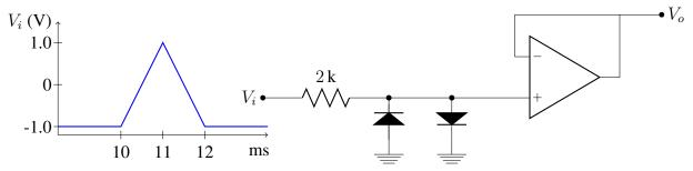
Sketch  $V_+$  and output  $V_o$ . Show voltage levels and the times of any transitions. (Assume op amps are ideal; diodes have  $V_D=0.7V$ )
