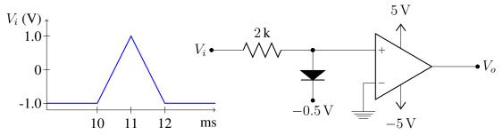
Sketch  $V_+$  and output  $V_o$ . Show voltage levels and the times of any transitions. (Assume op amps are ideal; diodes have  $V_D=0.7V$ )
