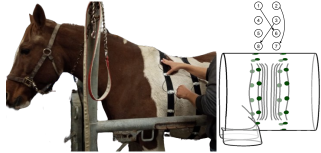
Fig. 1: Left: A horse with two-plane EIT electrode belts. Right: Electrode model sensitivity and stim/meas pattern.
