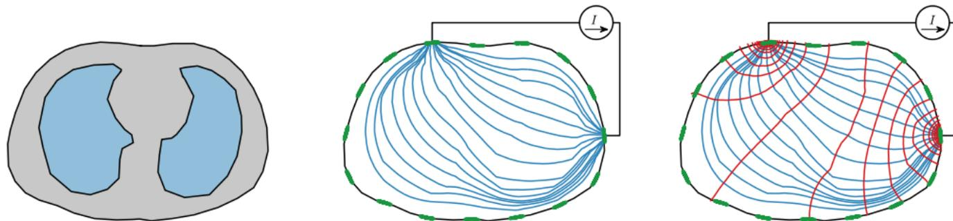
Electrodes on the body surface are used to inject current and measure the resulting voltages.
