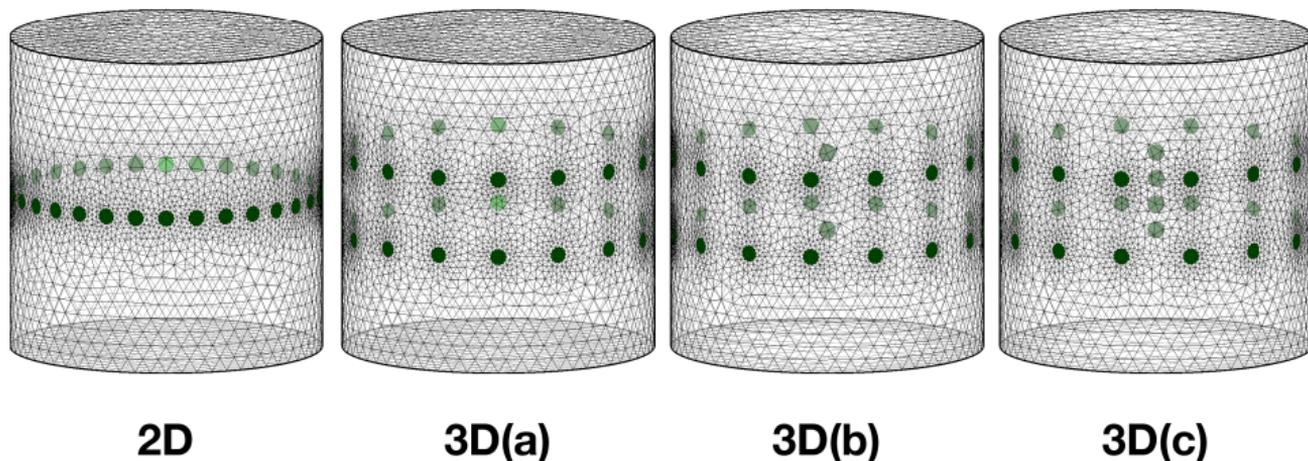
Typical 2D and 3D configurations are compared to internal electrode configurations.
