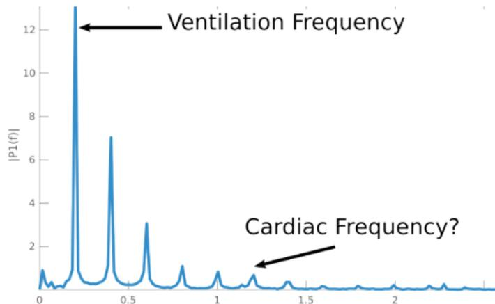
Example FFT of an EIT signal with only external electrodes (frequency in Hz).
