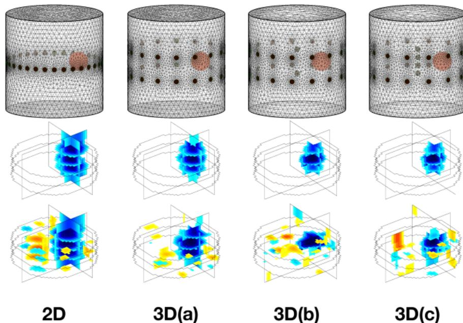
Internal electrodes were used to reconstruct the target closer to actual size.
