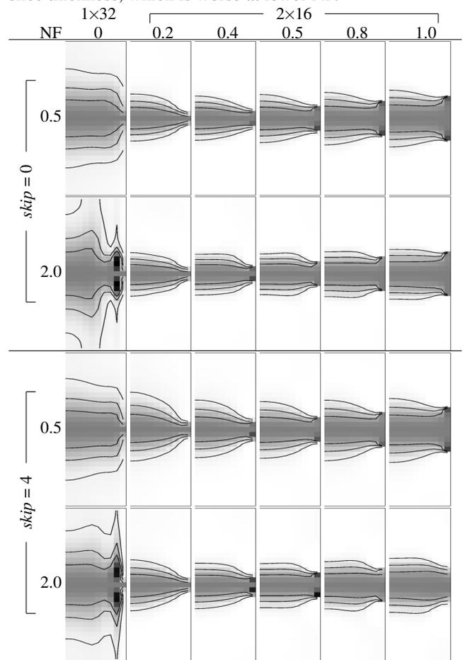
**Figure 3:** Normalized amplitude response (sum of in-plane image pixels divided by the value on the centre slice) for targets in the central sagittal plane. Each image has horizontal axis from centre to minor-axis side and vertical axis from  $h = -1.5$  to 1.5. Contours at 75%, 50% and 25% and only positive values shown.
