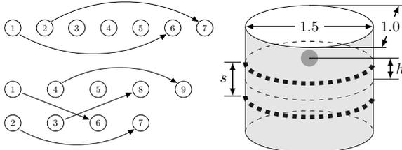
**Figure 1:** Left: One- and two-plane electrode configuration using the *square* pattern and *skip=4*; Right: Simulation geometry with electrode planes separated by  $s$  and a target  $h$  above the centre.
