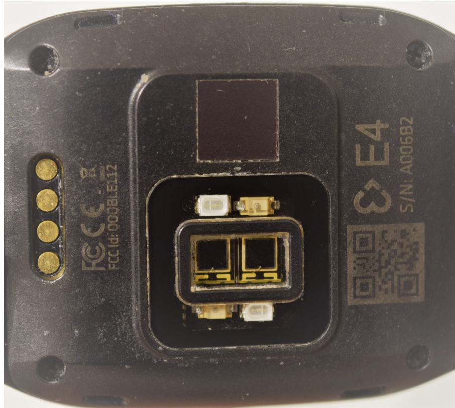
Figure 3.2: The Empatica E4 wristband’s PPG sensor consists of four LEDs and two photodiodes.
