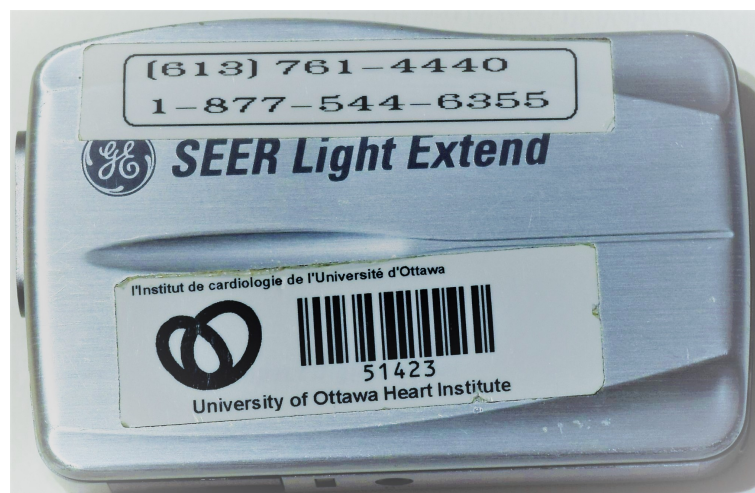
Figure 3.4: The General Electric Seer Light Extend Holter monitor was the source of the ECG Signal.
