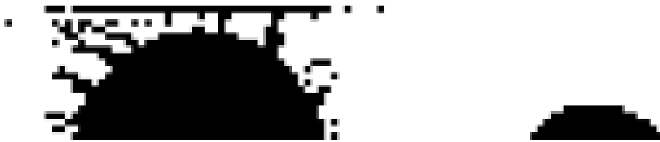
Figure 4.12: Example of a binary mask applied on the unwrapped iris image in the Masek's segmentation technique. The binary 0s (black pixels) indicate noise and are used to discard the underlying pixel values in the iris template. The pixel value corresponding to 1s (white) are used for the Hamming distance calculation.
