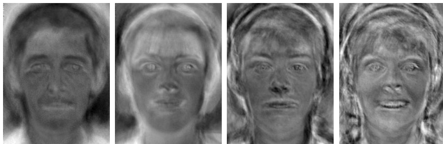
Figure 5.2: An example of FLD face features. From left to right, FLD features number 7, 10, 30, 50 are shown. FLD attempts to maximize class separation while minimizing the within class scatter.
