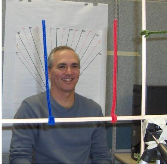
**Figure 3** Photo capture configuration: A subject in front of the photo capture and pose calibration apparatus. A camera tripod (shown) is placed at 2.0 m from the subject. For pose measurement, the subject wears a custom cap calibrated to point vertically. Each pose variation image is based on target lines as described.
