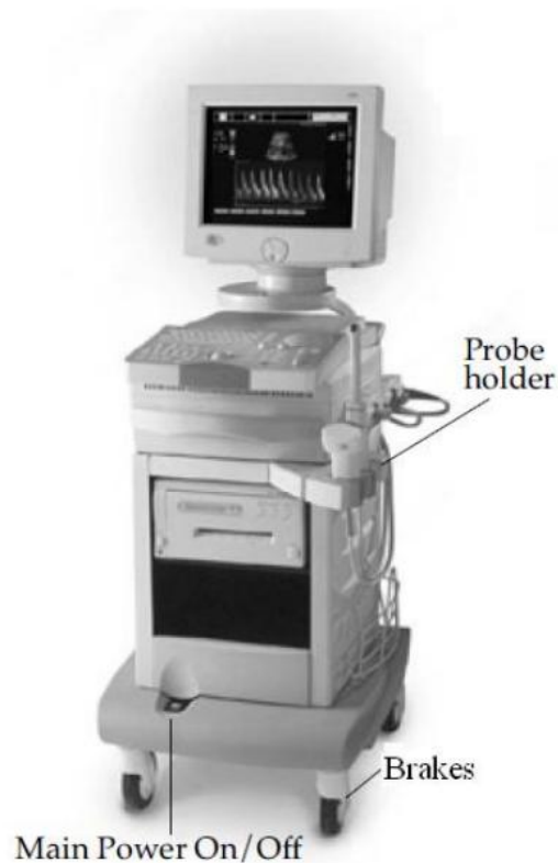
Figure 3.1 Picus ultrasound hardware. Reproduced from (Silver, 2009)
