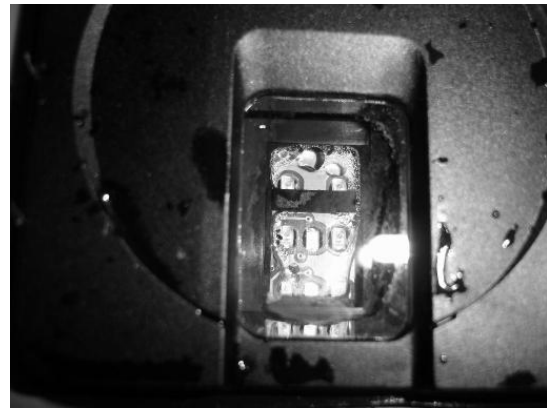
Fig. 10. Condensation build-up under optical scanner window.
