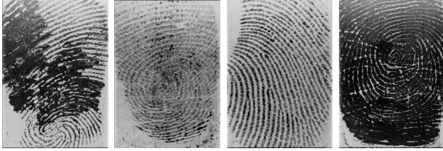
Fig. 5. Examples of rejected fingerprint images: (from left to right:) fingerprint covered with liquid; fingerprint moved during scanning (blurred image); fingerprint incorrectly placed; fingerprint applied with too much pressure (blurring features).
