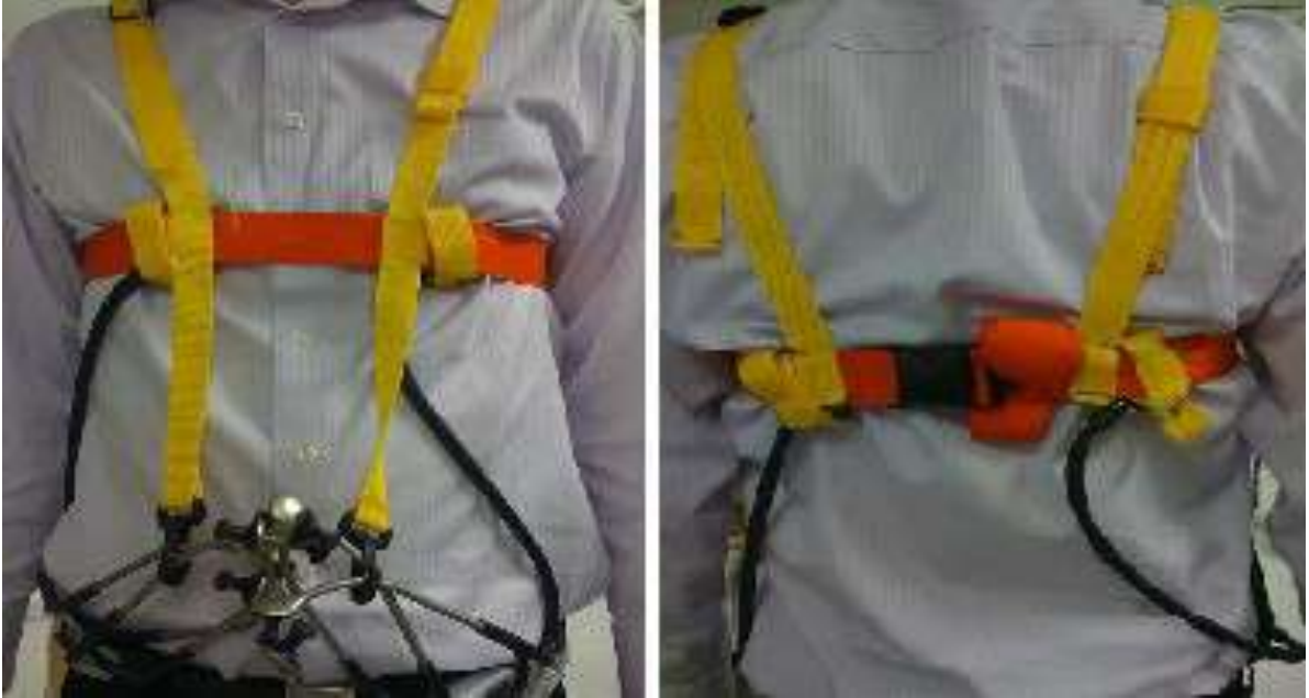
Figure 10 - Fully Adjustable Stethoscope Array Harness Attached to a Human Participant
