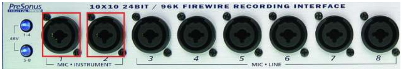
Figure 14 - Face Panel of Firepod Preamplifier. Boxes Show Channels 1 and 2 of the Preamplifier.
