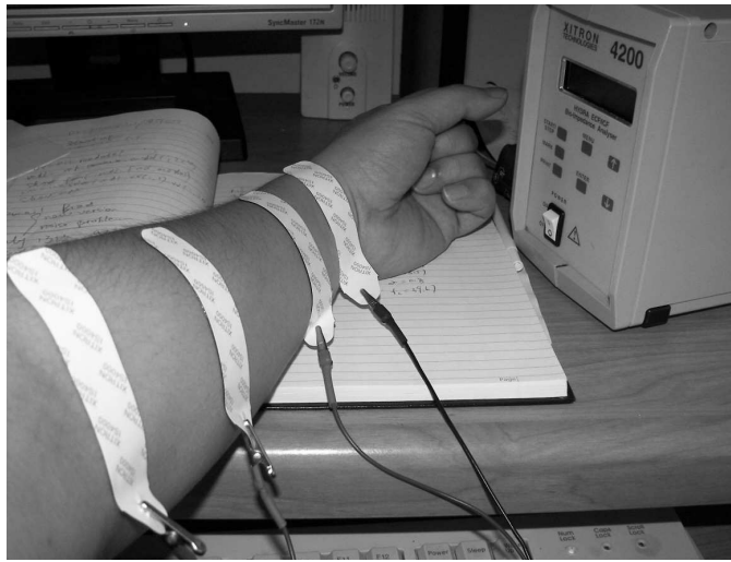
Figure 7.10: A preliminary blood pooling experiment on human arm. A tetrapolar BIS sensor applied on the forearm. Two impedance spectroscopic curves were obtained before and after blood pooling. The upper arm is clamped by a cuff of a blood pressure meter.
