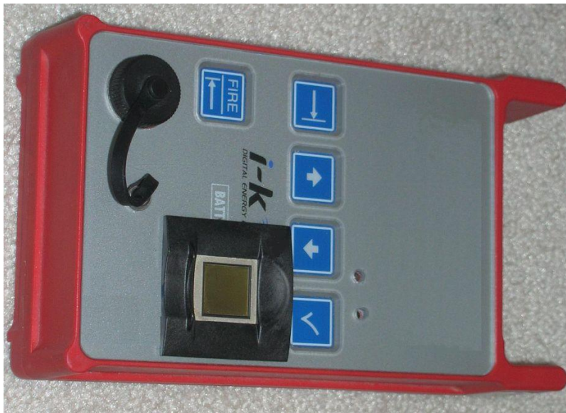
Figure 1: Fingerprint capture unit mounting on electronic blasting unit. The fingerprint sensor is shown at bottom left.
