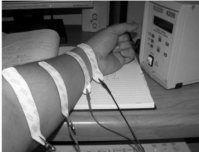
Fig. 10. A preliminary blood pooling experiment on human arm. A tetrapolar BIS sensor applied on the forearm. Two impedance spectroscopic curves were obtained before and after blood pooling. The upper arm is clamped by a cuff of a blood pressure meter.
