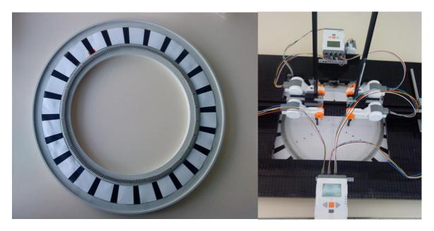
The whole system rotates on this grey ring. The black-white marks are for the Light-Sensor and the racks are for a gear on the actuation of the rotation.
