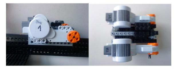
Carriage 3 and carriage 4 are identical but mirror inverted. Both use one motor for the x-movement and one motor for the z-movement. It uses gears to move on the x-axis as well as to move the z-axis with the object.
