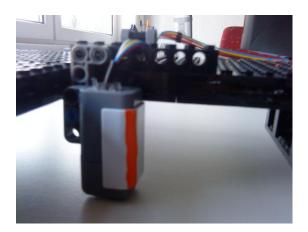
Use a construction like this to fix the light-sensor. It should be on the same side as the actuation of the rotation.
