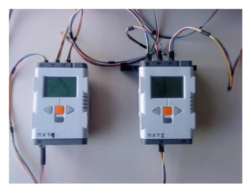
You will need two controllers to control the 7 motors. If you want to use the "EIT-P-PS" – program, you will have to load the programs "Prgm EIT-P-PS\_NXT1", "Prgm EIT-P-PS\_NXT2", "initialization\_nxt1", "initialization\_nxt2" to the NXTs. Unfortunately you will have to use the Bricx Command Center 3.3, which is freeware and can be easily find on the internet, for that. Make sure that you connect the cables to the right motors.
