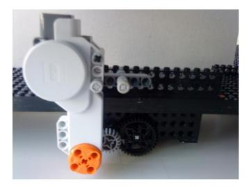
Fix one motor as above on the baseplate. Stick it on the axle so that the motor is able to rotate the whole plate.
