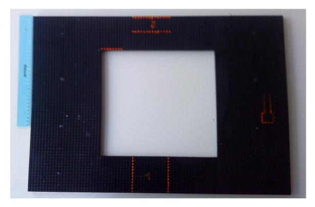
The baseplate of the EIT-Phantom-Positioning-System is, as all the other parts, made of LEGO. The size is 88x60 LEGO-pimples with a 40x36 hole in the middle. I won't count the bricks I have used to build this. Just use normal LEGO-plates with a height of 1/3 and stick it four-ply together.
