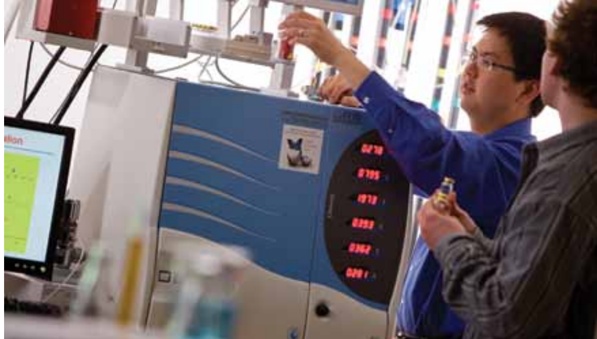
Professor Adrian Chan and his students examine whether food borne bacteria can be detected and identified by odour. Here, they prepare samples to be tested by an electronic nose.
