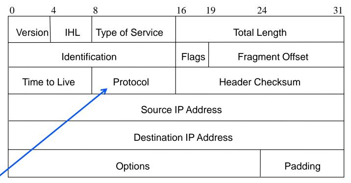
**Protocol:** specifies **upper-layer protocol** that is to receive IP data at the destination. Examples include TCP (prot. = 6), UDP (prot. = 17), and OSPF (prot. = 89).
