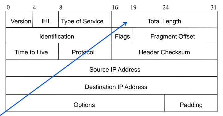
Total length: number of bytes of the IP packet including header & data (payload), maximum length is 65535 bytes.
