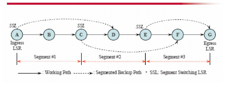
When a fault is detected, the fault notification needs to propagate to the Segment Switching LSR (SSL) of that domain instead of the ingress LSR
