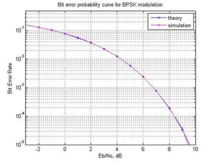
Consider an LTE application that uses BPSK modulation; the corresponding BER versus SNR  $(E_b/N_0)$  relation is given in the above figure. This application requires a BER of  $10^{-4}$  and it is assigned one RB.
