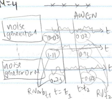
AWGN  $\rightarrow$   $R_{V_{t_1}}, R_{V_{t_2}}$ : Gaussian RV
