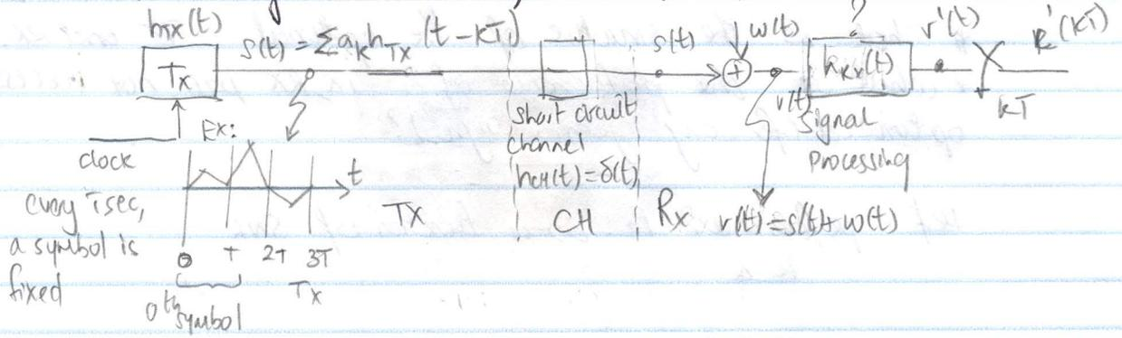
Meaning of M-ary PAM - Pulse Amplitude Modulation
