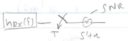
Meaning of MF =  $h_{rx}(t) = h_{rx}(T-t)$  — Matched filter
