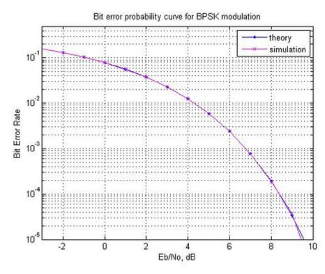
Consider an LTE application that uses BPSK modulation; the corresponding BER versus SNR ( $E_b/N_0$ ) relation is given in the above figure. This application requires a BER of  $10^{-4}$  and it is assigned one RB.
