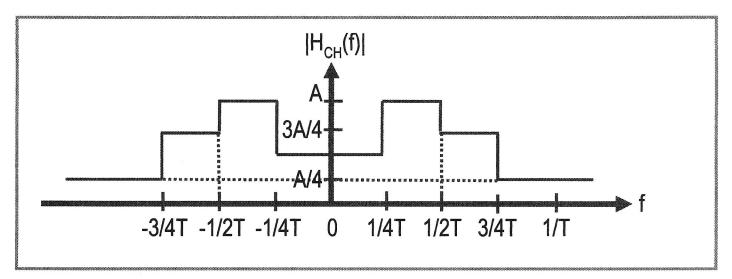
Sketch the equalizer transfer function (magnitude) which will completely remove the effect of the channel yielding a no-ISI situation.
