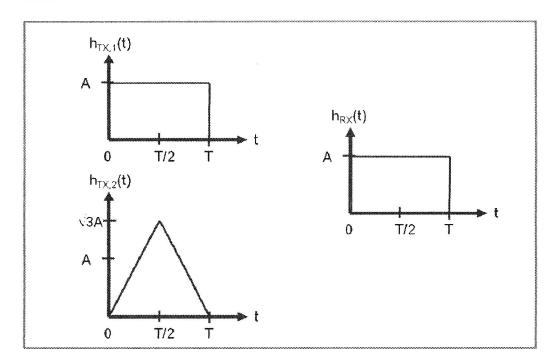
The transmitter pulse shaping filter impulse responses are given above for two different schemes, along with the receiver filter impulse response which is the same for both schemes. Clearly, the receiver is not matched to the transmitter in Scheme 2.
