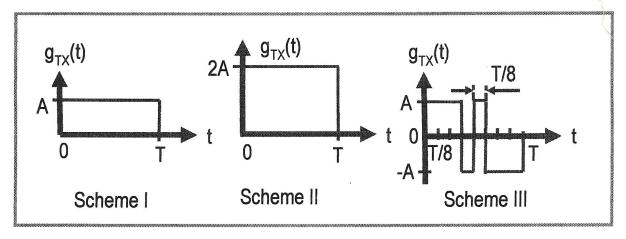
It is given that the bandwidth of Scheme I is 3.2 MHz.
