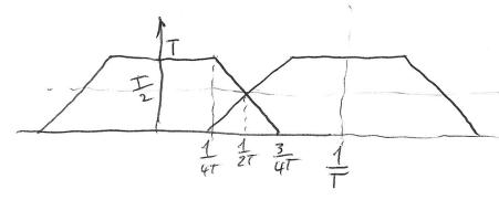
b) If the TX and RX filters are designed as matched filter pairs under the assumption that the channel is perfect (i.e.,  $h_{CH}(t) = \delta(t)$ ), sketch  $|H_{TX}(f)|$  and  $|H_{RX}(f)|$ . 15 pt
