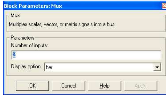
Figure 19: Block parameters for the Mux block.
