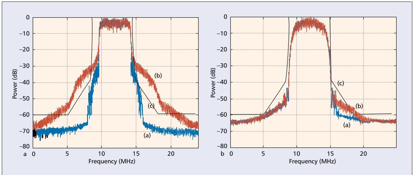
**Figure 1.** a) Power amplifier output power spectra [5] for a QPSK 256-point OFDM system: (a) spectrum with ideal power amplifier (infinite power backoff); (b) spectrum with typical power amplifier with 10 dB power backoff; (c) FCC MMDS spectral mask; b) power amplifier output power spectra [5] for a QPSK SC system: (a) spectrum with ideal power amplifier (infinite power backoff); (b) spectrum with typical power amplifier with 10 dB power backoff; (c) FCC MMDS spectral mask.
