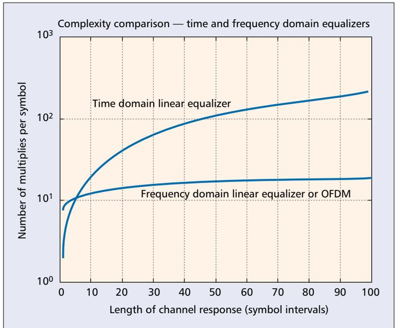
■ **Figure 4.** Complexity comparison of time and frequency domain linear equalizers with LMS adaptation.
