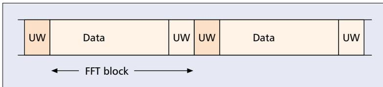
■ **Figure 8.** Continuous downstream transmission showing unique words (UW) used for training shaded.
