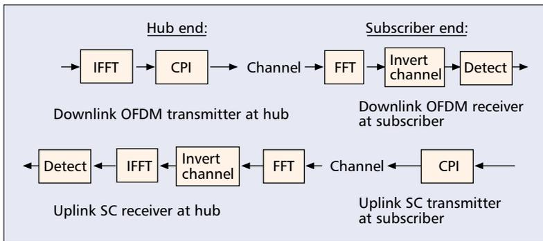
■ **Figure 7.** Coexistence of SC-FDE and OFDM: uplink/downlink asymmetry.
