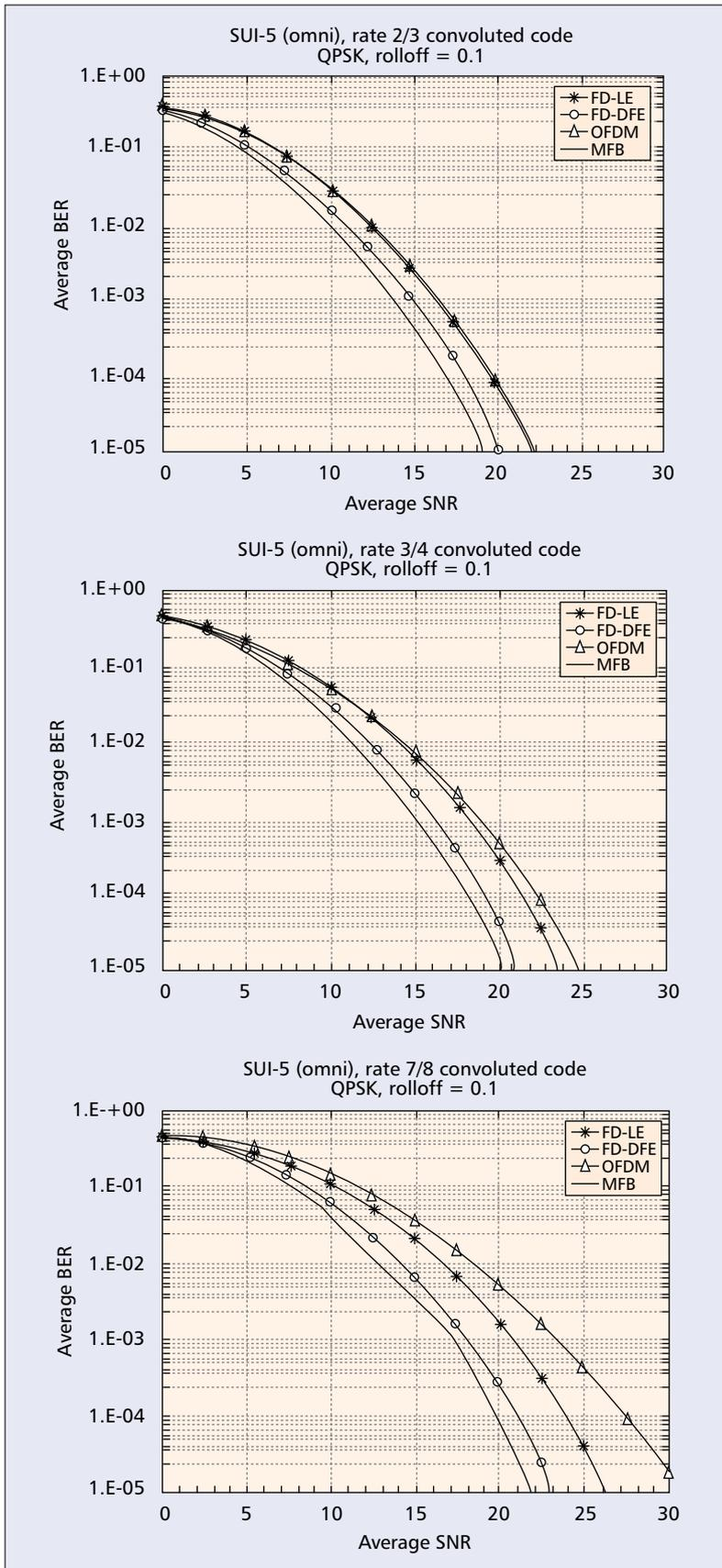
**Figure 11.** a) Performance comparison for systems with perfect channel knowledge on SUI-5 channel model for QPSK with code rate 2/3; b) performance comparison for systems with perfect channel knowledge on SUI-5 channel model for QPSK with code rate 3/4; c) performance comparison for systems with perfect channel knowledge on SUI-5 channel model for QPSK with code rate 7/8.
