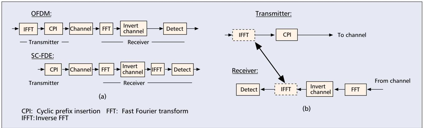
■ **Figure 6.** a) OFDM and SC-FDE — signal processing similarities and differences; b) potential interoperability of SC-FDE and OFDM: a "convertible" modem.
